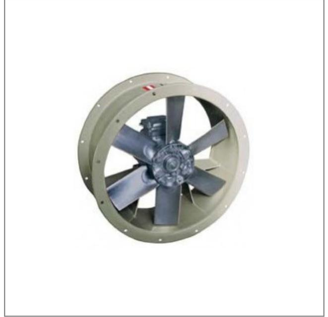
Côte d'encombrement : ØA= 810mm, ØB = 770mm, ØD = 710mm, E = 430mm, ØJ = 12mm, N = 16x22°x30'
