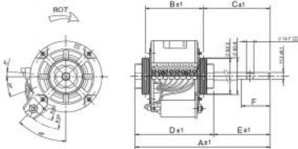
Cote d'encombrement : A = 318,1mm, B = 100-124mm, C = 189-201mm, D = 136,2mm, E = 181,9mm, F = 110mm
